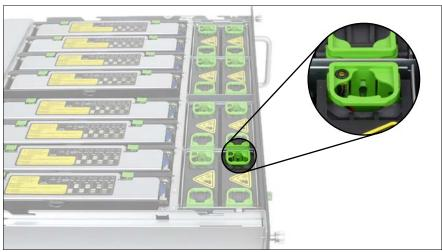
Figure 21: Indicator on a hot-plug fan
